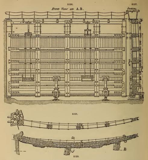
1 ft. 7 in.; third post, 1 ft. 5 in.; and mitre-post, 1 ft. 2 in. The cross-pieces are curved on the side of the pressure, but straight on the other side between the posts with which they are flush. It follows from this diminution of thickness towards the top that the radius of curvature, which is  $96 \cdot 4$  ft. at the bottom, is about 124 ft. at the top, in consequence of the flattening of the leaf.
